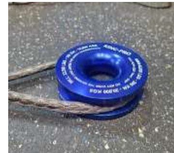
Snatch Block / Pulley- Rope Ring – made from steel or aluminum, use a hard or soft shackle on block but only a soft shackle on a rope ring
