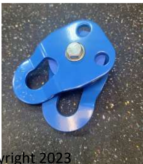
Snatch Block / Pulley- Rope Ring – made from steel or aluminum, use a hard or soft shackle on block but only a soft shackle on a rope ring
