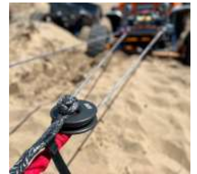
Snatch Block / Pulley- Rope Ring – made from steel or aluminum, use a hard or soft shackle on block but only a soft shackle on a rope ring
